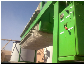
625 Liter Semi-Automatic Filter Press Ceramic Industry Waste Treatment Plant 6 th of October Industrial City
