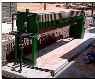
160 Liter Semi-Automatic Filter Press Metal Finishing Waste Treatment 10 th of Ramadan Industrial City
