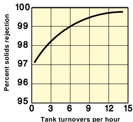
Hydraulics indicate a turnover rate of 14 times is required to have all the liquid pass through the filter once.
