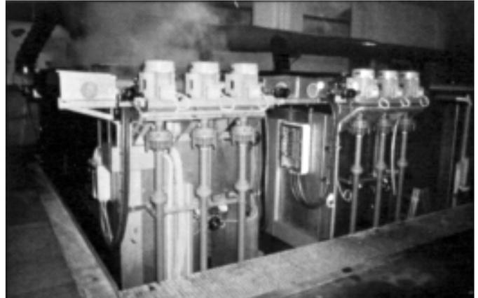
*EN SOLUTIONS can be filtered using out-of-tank vertical centrifugal cantilevered seal-less pumps, as in this installation.*
